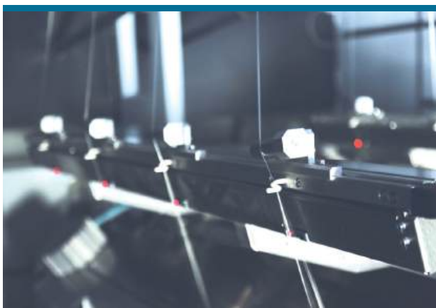
The ACW high-speed winder processes HMLS yarn at speeds of up to 6300 m/min.
