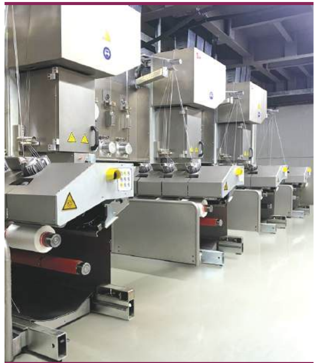
The three-end BCF system BCF S+ is extremely flexible: even in the design optimized for polyester yarn production, the system produces excellent polyamide 6 yarn
