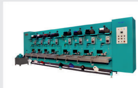
Single End Sizing RI 8001 (1-4-8 Spindles / Speed 250 MPM)
