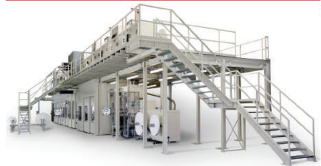
W+D BICMA feminine care products manufacturing machine
