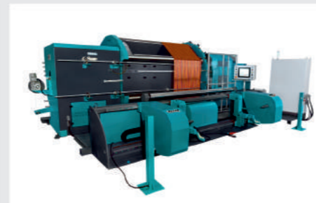
High Speed Automatic Sample Warper RI 6001 (220 cm / 27-500 meter / 16 colours)
