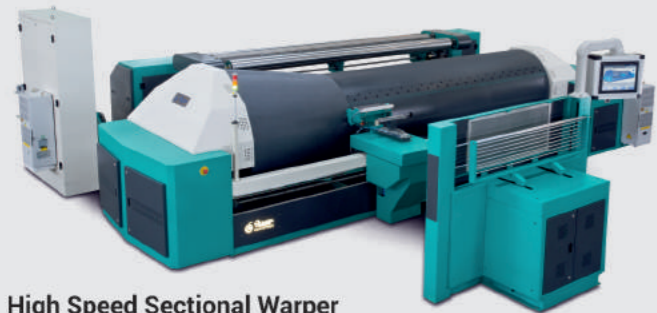
High Speed Sectional Warper Maximum Warping Speed : 1000 mtr/min Maximum Beaming Speed : 200 mtr/min
