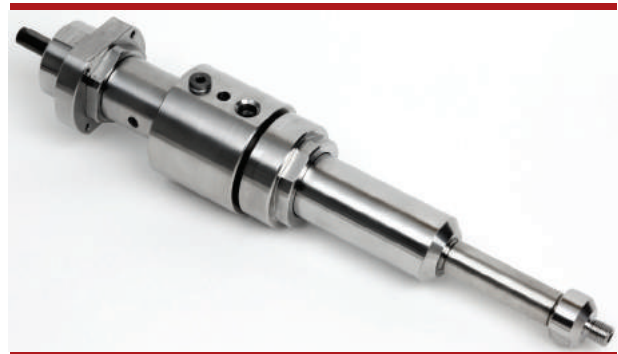
The series of eccentric screw pumps covers a throughput range of between 1 ml/min. and 30 l/h, also conveying – with viscosity range of between 1 mPas and 1,000 Pas – highly-filled, high-viscosity or even abrasive media.
