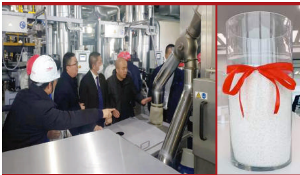
The PBS system at Yingkou Kanghui Petrochemical Co. Ltd. was production-ready within just 14 months. Initially, the company will use the new equipment to produce the biodegradable copolymer polybutylene adipate terephthalate (PBAT).
