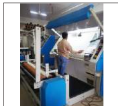
Classic Inspection & Rolling behind operator
